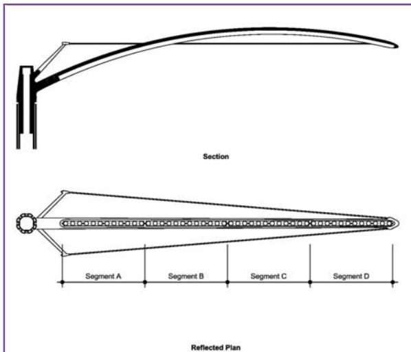
Diagram of the LED luminaire seen from the side and below
