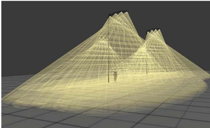
Ray trace diagram of the double column's light distribution.
